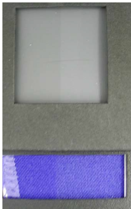
Photo 1: Blue wool reference swatches after exposure No 5 (bottom) grey scale reference 4 (above). Right hand side shows exposed region.
