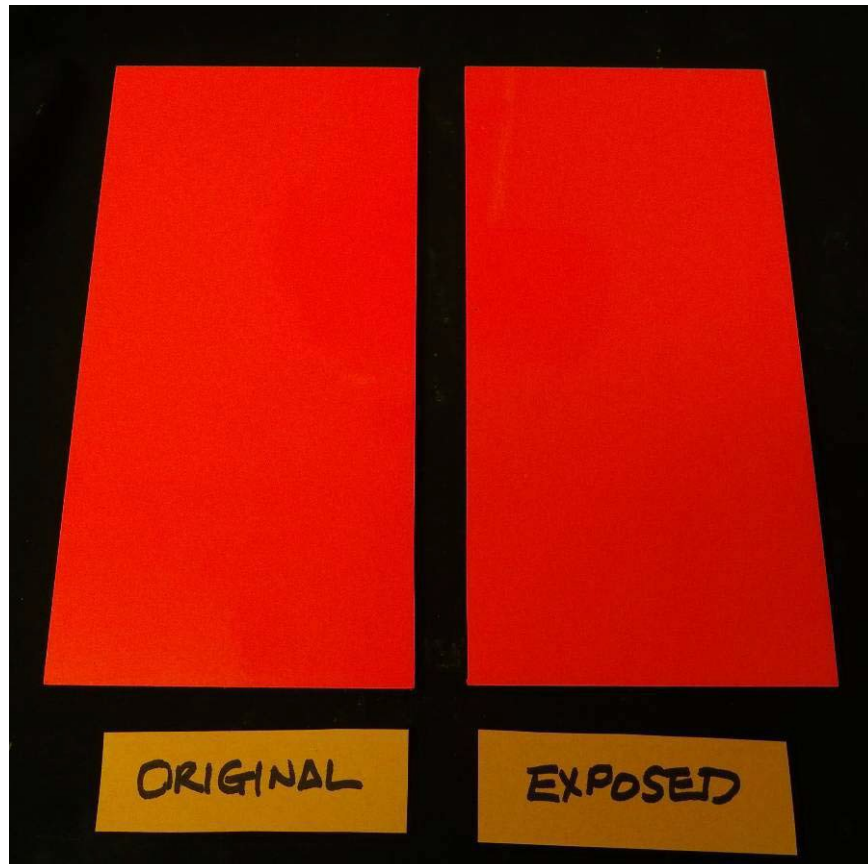
Photo 3: Sample S2 – Unexposed on left and exposed sample on right. 43 hours of UV exposure.
