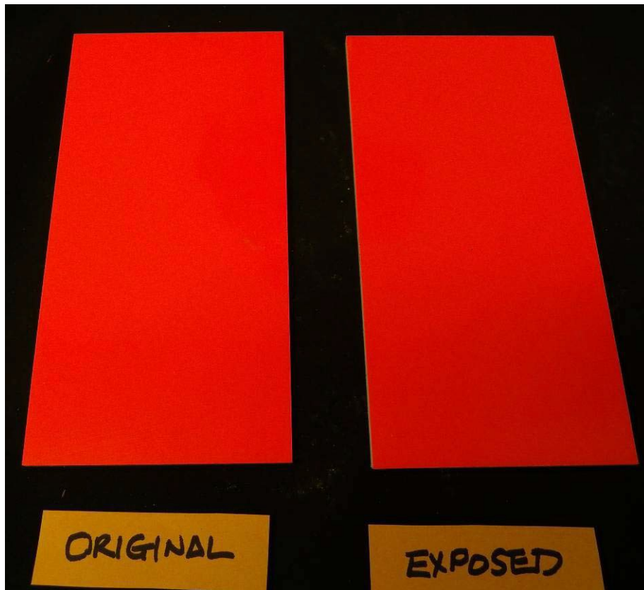
Photo 2: Sample S1 – Unexposed on left and exposed sample on right. 43 hours of UV exposure.
